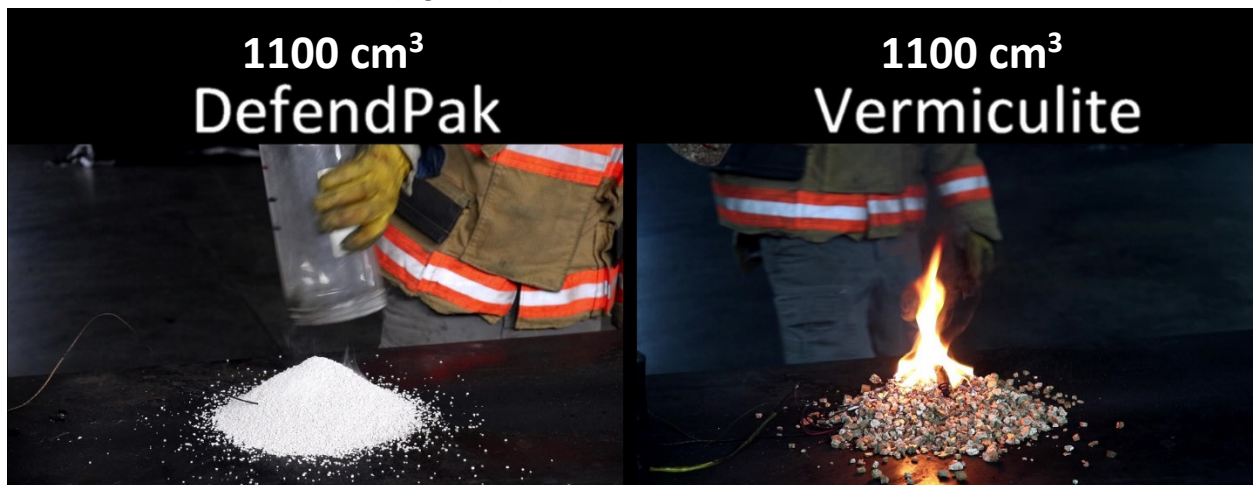
Figure 2. LIPO battery pack tests after 1100 cubic centimeters of media has been applied.
